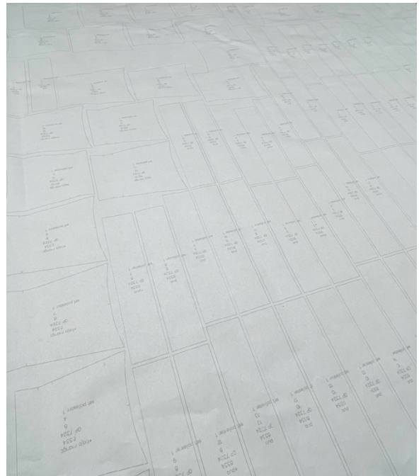
Figures 38 & 39 – Marker used to identify cut parts; the information shown in the paper: Article Number; Size; Number of parts for that size; PO number; Type of fabric.
