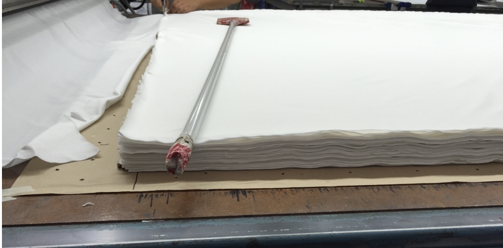
Figure 34 - Ply of fabric after spreading process.
